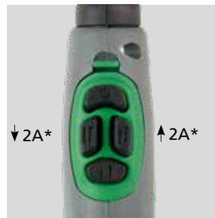
Up/Down module with 4-function key for adjustment of welding current incl. TIG-A Tack function. The welding current is increased / reduced with 2 amps. Long press for constant increase / decrease. Art. no. ....80300063
