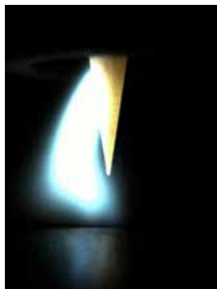
Low-quality tungsten: typically sideways arc ignition. the arc flashes and wanders slowly to the electrode tip which has to be cut off and reground.
