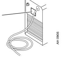
**Note!** The welding power source is designed for connection to a 400 volt system with four conductors. If the power source is to be used in countries with a higher or lower supply voltage, the power source must be connected via a safety transformer.
